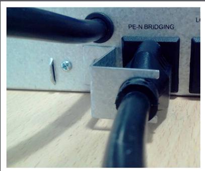
**AC input plug and Z plate should not be removed from the PE-N bridging when inverter is running.**
